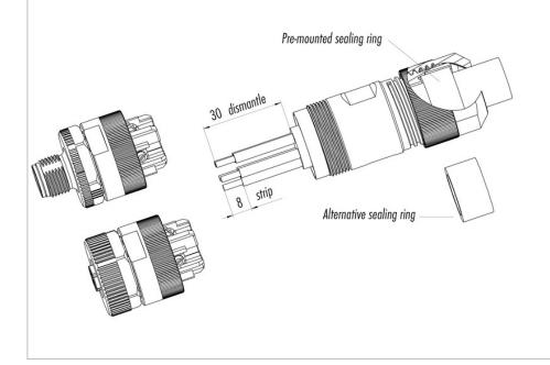
1. Clamp out screws until bores for single wires are completely free.
